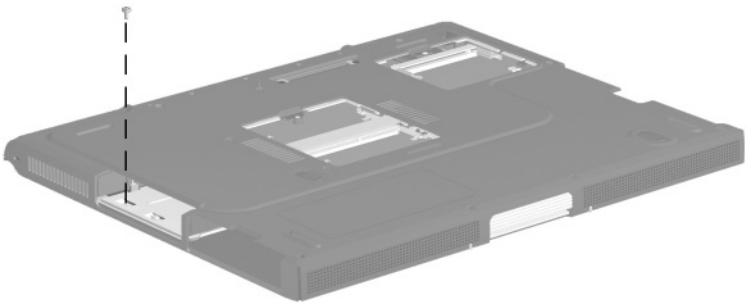
Figure C-8. Phillips M2.0 × 4.0 Screw Locations
